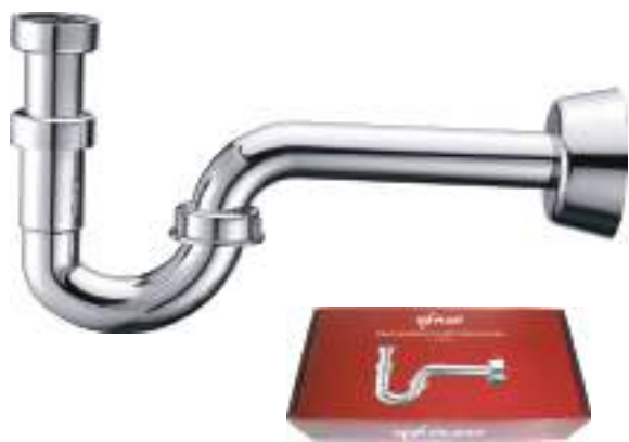
Sifone minimalista a "P" in ABS cromato per lavabo 1"1/4 Chrome plated ABS "P" siphon 1"1/4
