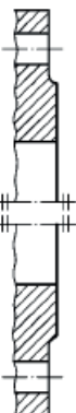
Tipo / type B Tenuta a gradino (B1 e B2) Raised face (B1 and B2)
